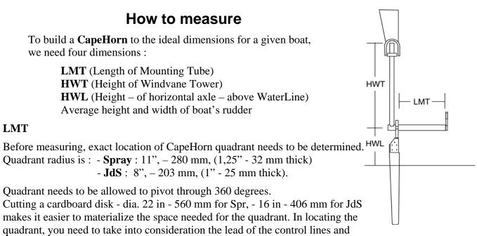
the location of the first pair of turning blocks, which need to be in line with the groove in the quadrant.
