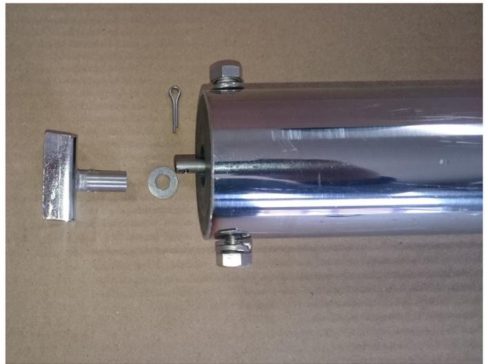
2 : Pull the two screws fastening the  $1\frac{1}{2}$  in. bushing that supports the aft end of the rod. Mark the precise position of the bushing (see below) Pull the rod with the bushing aft.
