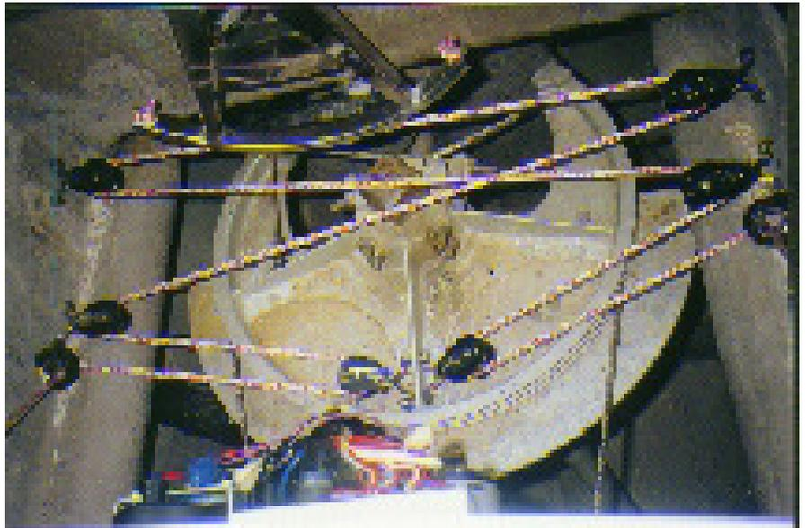
**CH** quadrant mounted down. Lines connected direct to blocks fastened to circular quadrant, pulling from aft of the rudder stock. (Christina 40).
