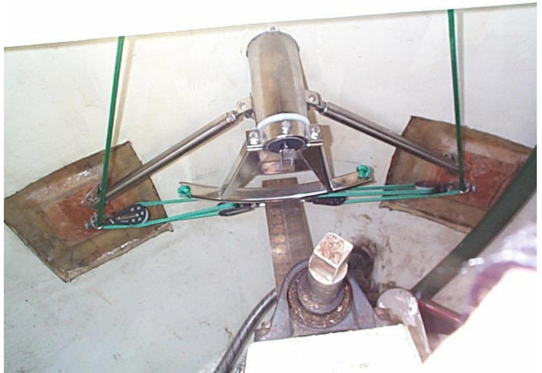
**CH** quadrant mounted down, lines connected forward of the rudder stock have to be crossed. (Bénéteau Oceanis 39).
