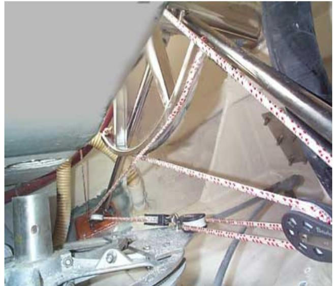
(Seen from above) Axle offset to locate **CH** quadrant in front of rudder stock ; control lines led to block on tiller (which has **been** extended) to which hydraulic ram is connected. (CT 37)
