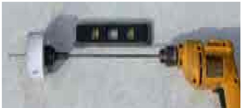
The secret is to maintain the tool very steady, level and parallel to the centre line; this way, you will easily cut through the transom, even if it is at an angle. Or through the curved surface of a canoe stern. If the drill is held very steadily, the hole-saw will not bind. If possible, cut half the thickness from the outside and half from the inside.
