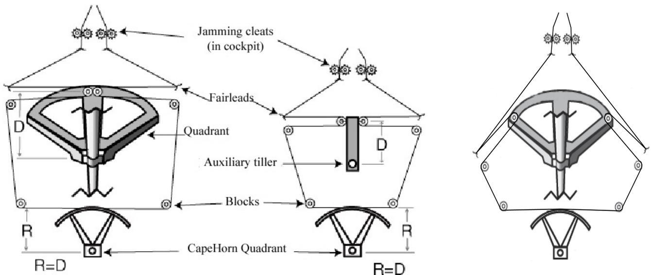
**Note** : when the vane is in operation, only the segment of control lines between the two quadrants (or CapeHorn quadrant and aux. tiller) moves and therefore, needs to be led through blocks. The segment between the rudder quadrant (or tiller) and the jamming cleats does not move, it is only kept in tension and can be led through fairleads instead of blocks.
