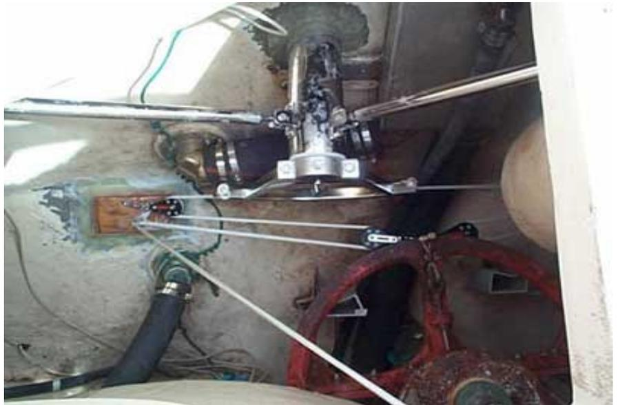
**CH** quadrant mounted down. Lines led to blocks fastened to pads bonded to the hull. Lines look like they are crossed, but actually, they are not : they pull directly from the other side of the steering quadrant. (Union 36).
