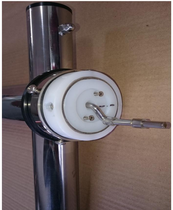
3 : Remove the  $\frac{1}{4}$  in. fore-and-aft bolt at the top of the servo-pendulum stock. Pull the stock down.
