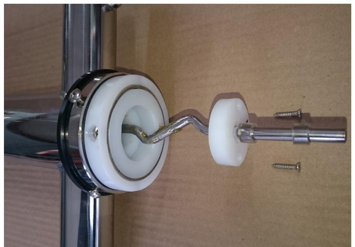
When re-assembling, the precise position of the co-axial control rod , both fore-and-aft and lateral, is critical to ensure that there is no friction between the control rod and the stock of the servo-pendulum.
