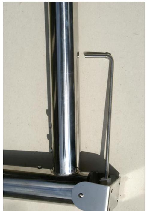
At the end of the autopilot ram, there is a hole made for connecting a vertical pin on the tiller. Turn the ram ¼ turn, drill this hole all the way through with a ¼ in. drill, and insert the L-shaped rod through this hole. Insert the dovetail-shaped plastic connector at the other end of this rod into the corresponding piece, at the end of the horizontal control axle.
