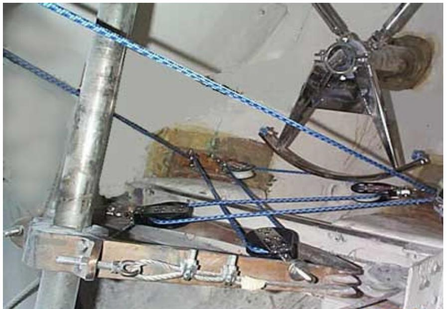
**CH** quadrant below axle, lines led to blocks on plate bolted to back of steering disk (CS36)
