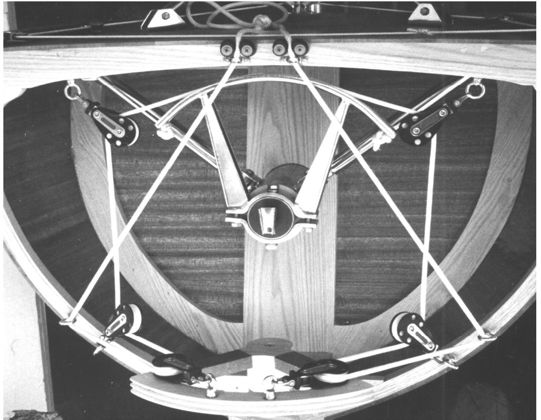
**CH** quadrant below axle, control lines led to blocks fastened on a short auxiliary tiller clamped on rudder stock (Pan Oceanic 43).
